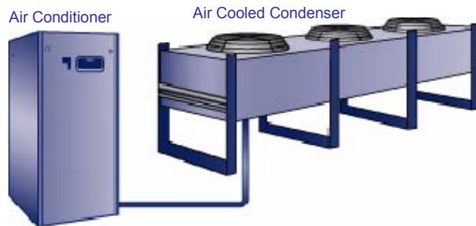
Figure 5 – Air cooled system
